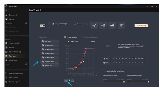
5. Configure the fan rpm curve to be controlled via the GPU temperature, deselect the CPU temperature control.
